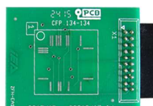
"ZFH-EA10" 64 Pins MCU PCB ADAPTER (08AZ/AB, 908AS/AZ)
