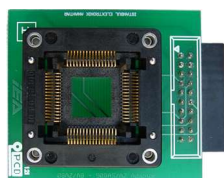
"ZFH-EA9" 64 PINS MCU ADAPTER WITH SOCKET
