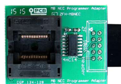
"ZFH-MBNEC" MERCEDES-BENZ KEY MCU NEC ADAPTER
