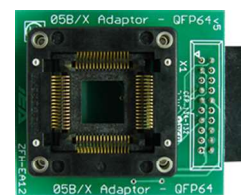
"ZFH-EA12" 64 PINS MCU ADAPTER WITH SOCKET QFP64(05B/X)
