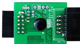
"ZFH-PCF79XX" REMOTE UNLOCKING ADAPTER
